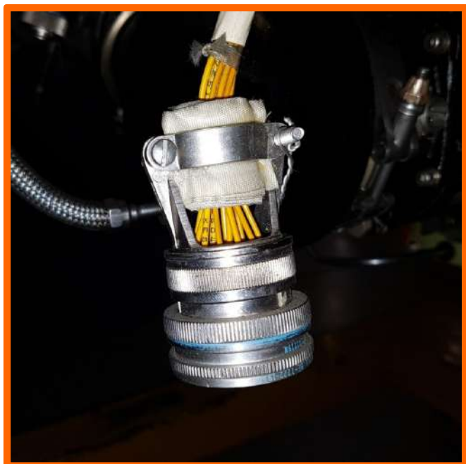
Tape used as a backshell clamp bushing
